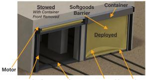
Manual Release Interface Step Gate Guide Seal Bar R072524
